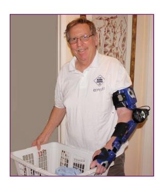
Sensors in the brace detect weak muscle signals, which power the motor to move the arm in the desired direction. The user is completely controlling their own arm; the brace simply amplifies the users weak muscle signal to help bend and move the arm. With the brace, a user is able to stabilize themselves to safely perform activities of daily living such as feeding, reaching, and lifting.
